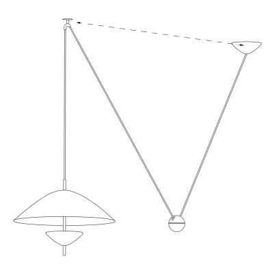
Measure the distance you want between the ceiling bracket and the canopy. Make sure the counterweight sphere is not in the way. Mark the position of the canopy.
