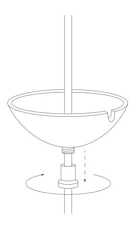
Unscrew the rod at the bottom of the canopy and remove the canopy cover.
