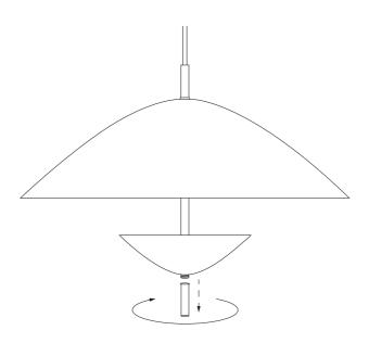
Unscrew the rod at the bottom of the lamp and remove the cover.
