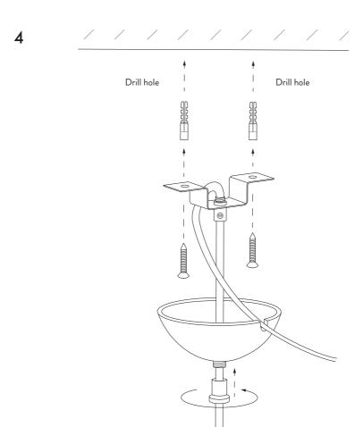
Drill the holes for the rawplugs then install the canopy bracket into the ceiling, make sure that the cable is well positioned in the slit. Secure the canopy cover by screwing it back.
